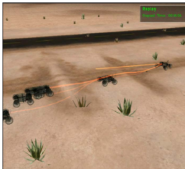
Figure 12: ANVEL Visualization Showing Repeated UGV Mobility Study. The "trails" show paths taken, with a UGV "ghost" remaining where the vehicle could
